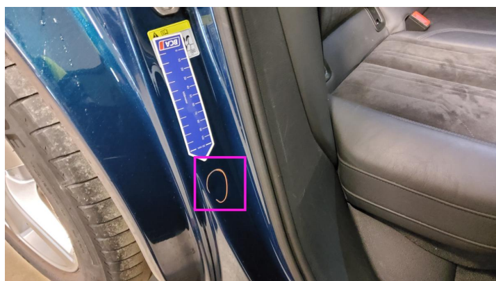
6. Door Step / Back Right Interior / Dented
