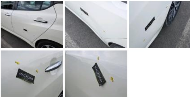
Aile ARG, Griffe(s), Acceptable
